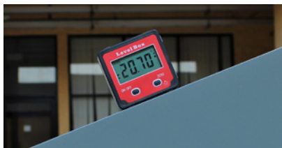
Fig. 20 Inclinometer used to verify that the upper edge of the gnomon formed an angle of 20.7^\circ with respect to the horizontal plane.
