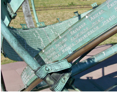
Fig. 6 Equatorial sundial 3.4 meters in diameter installed in Frankfurt, Germany, in 1951 (Loske 1999). Its dials mark the solar time of Frankfurt and the solar time of the 15° E meridian, which governs the legal time in Germany. It is also possible to determine the date, solar time , mean solar time and legal time of 200 cities around the world. The same can be achieved for any site on Earth, as long as its geographical coordinates are known. Design: Lothar M. Loske.
