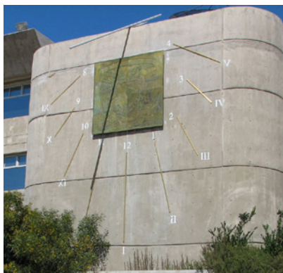
Fig. 5 Vertical declining sundial with a 3.3 meter gnomon installed at the Center for Nanosciences and Nanotechnology of UNAM in Ensenada, BC. The wall where the clock was drawn is not oriented exactly to the south but declines more than 8 degrees to the east, which is why the lines of the hours are not symmetrical. Design: Roberto Machorro.
