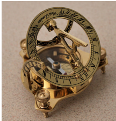
Fig. 7 Portable sundial made of brass (approximately 10 cm in diameter). Solar time can be determined by orienting the gnomon with the compass and adjusting the angle of dial.
